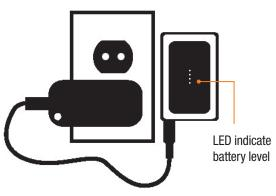
**LED light blinking =** Battery charging **Constant LED light =** Battery fully charged
