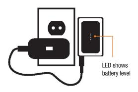
Red light – Battery charging Green light – Battery fully charged
