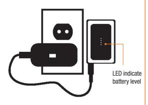
Red light – Battery charging Green light – Battery fully charged
